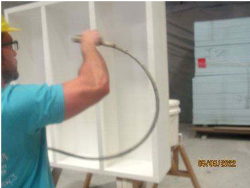
Photo No. 8 Spraying final coating
