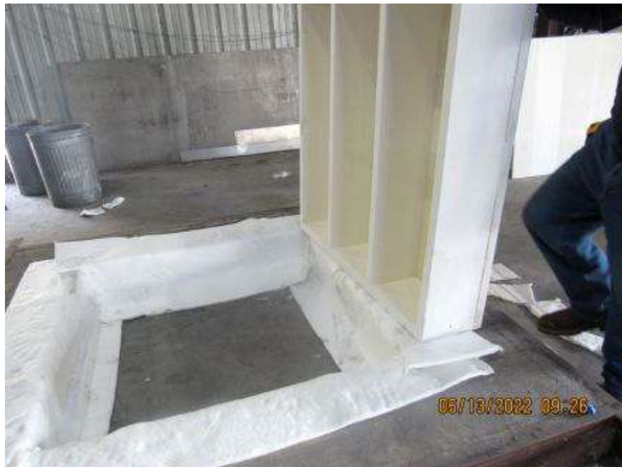
Photo No. 10 Installing assembly into test frame
