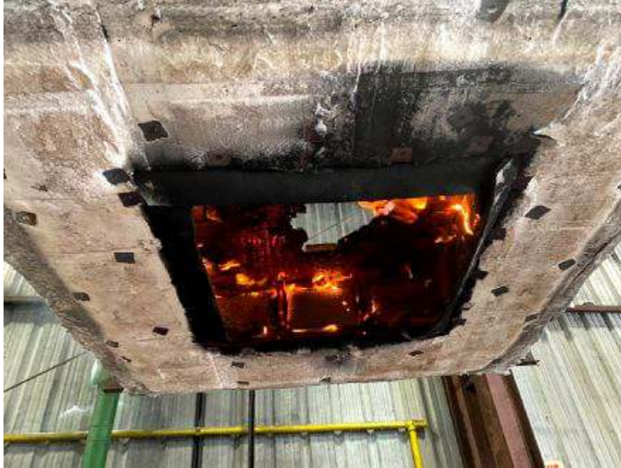
Photo No. 23 Exposed side flaming
