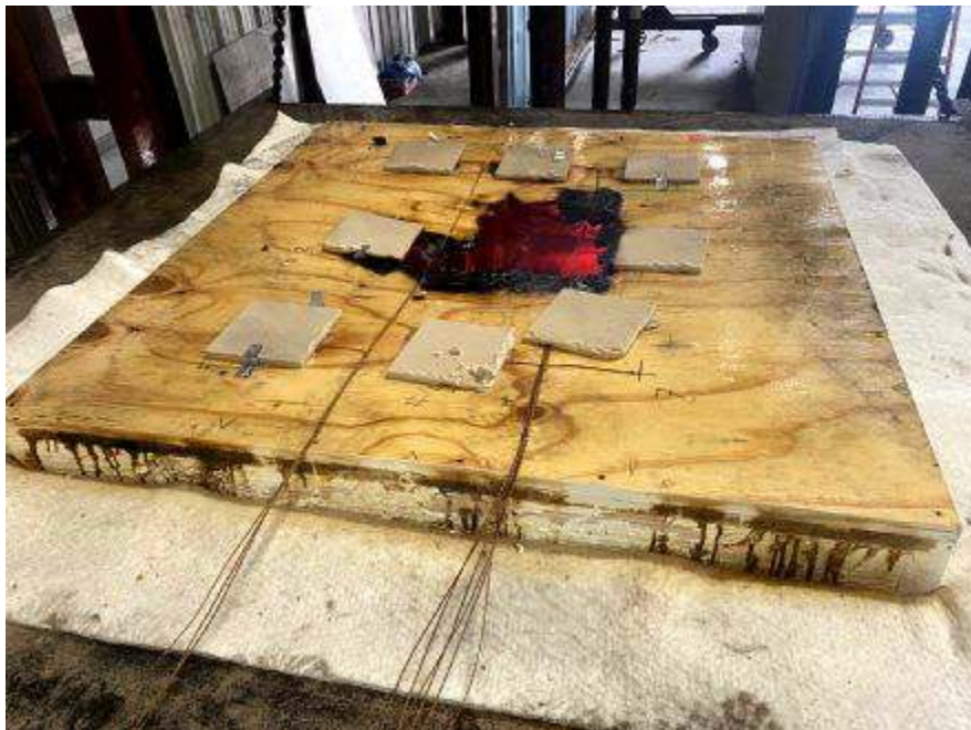
Photo No. 22 Hole burned through sample
