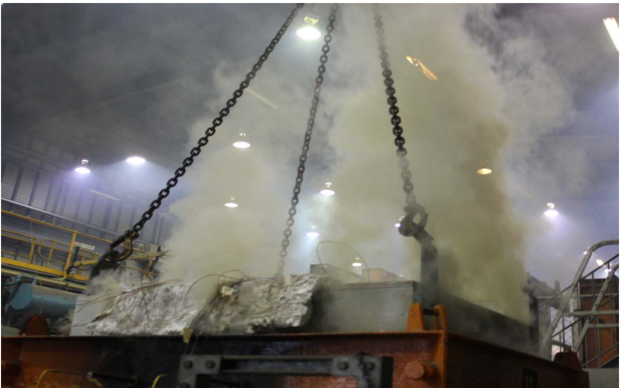
PHOTOGRAPH 6 – UNEXPOSED FACE OF SPECIMEN AT THE CONCLUSION OF TESTING
