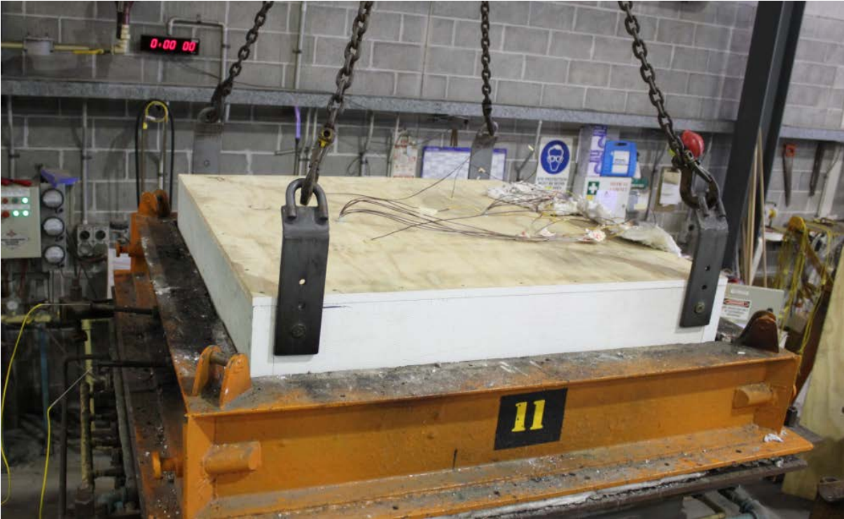
PHOTOGRAPH 2 – UNEXPOSED FACE OF SPECIMEN PRIOR TO TESTING
