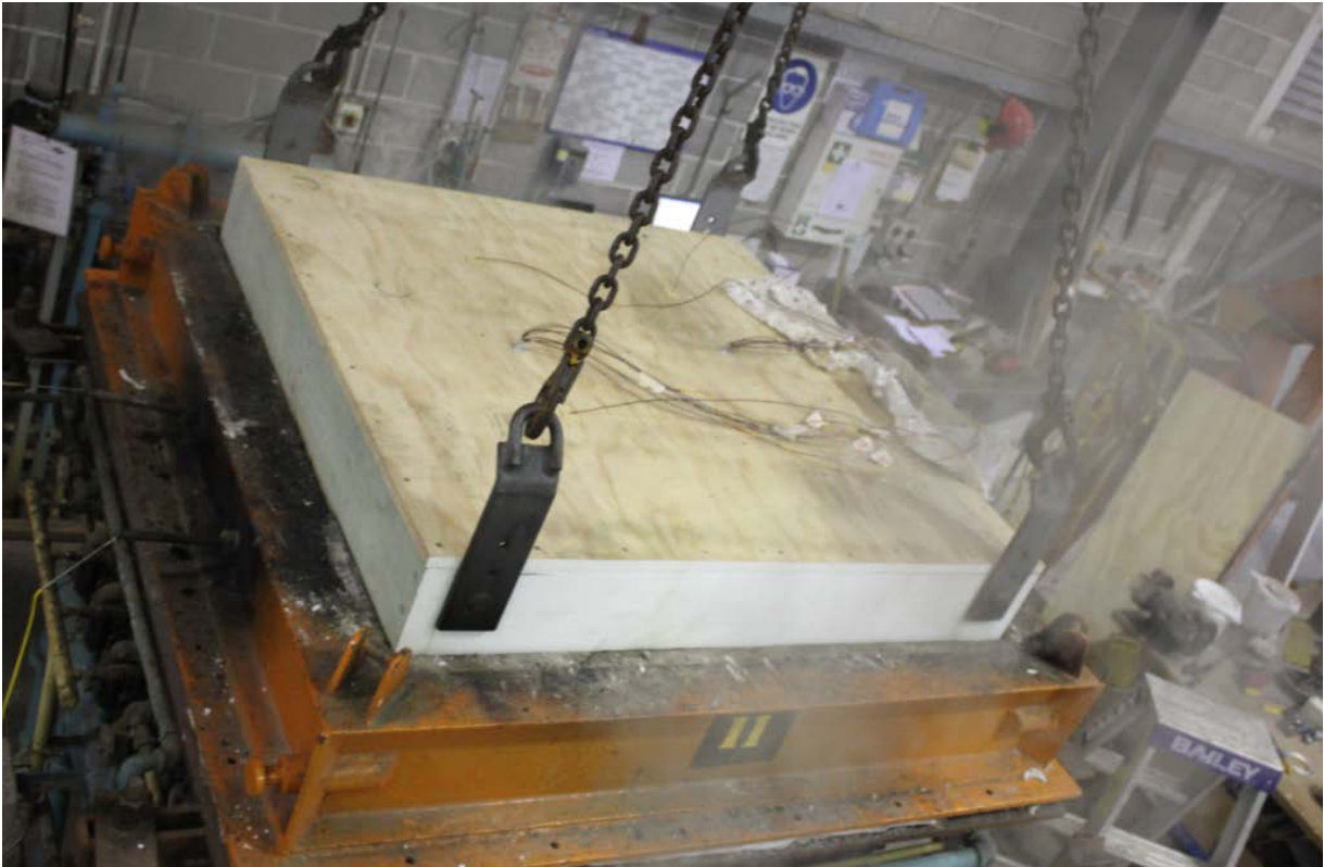
PHOTOGRAPH 5 – UNEXPOSED FACE OF SPECIMEN AT THE CONCLUSION OF TESTING
