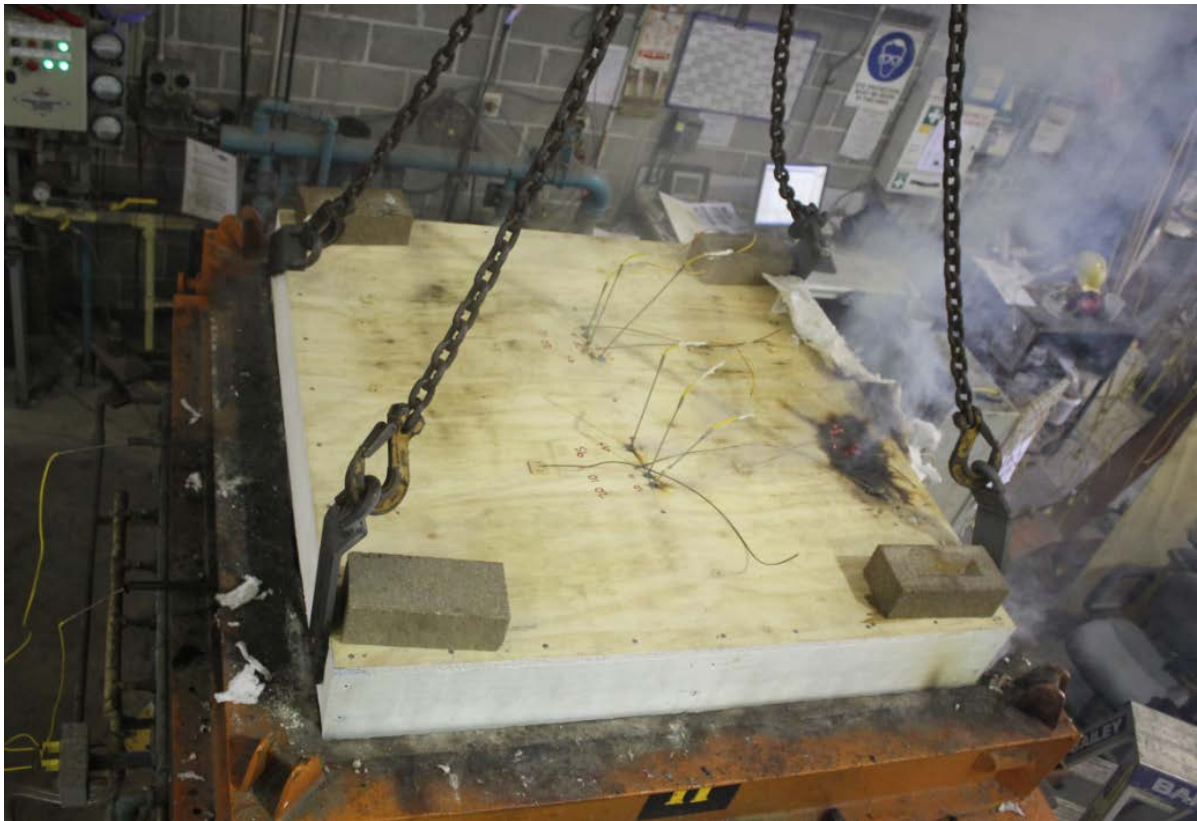
PHOTOGRAPH 5 – UNEXPOSED FACE OF SPECIMEN AT 50 MINUTES - CONCLUSION OF TESTING
