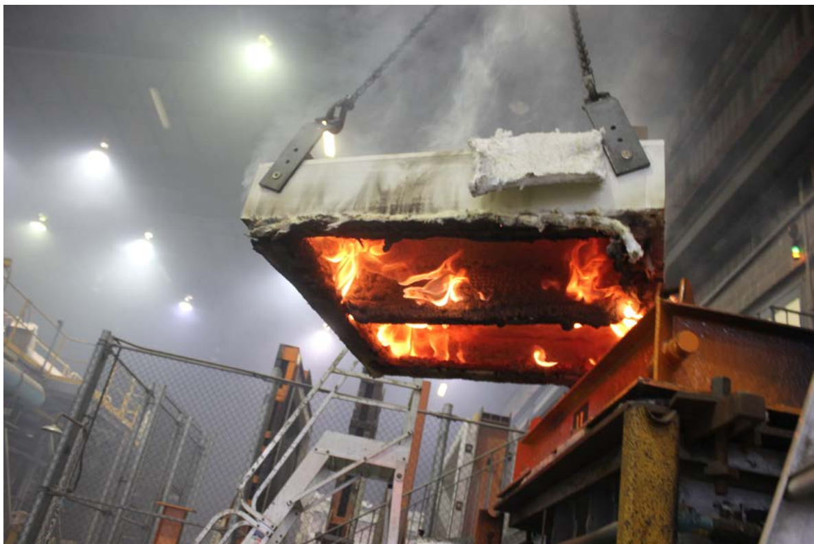
PHOTOGRAPH 6 – EXPOSED FACE OF SPECIMEN AT CONCLUSION OF TESTING
