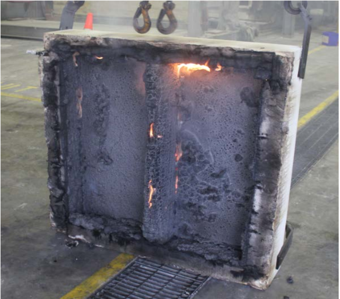
PHOTOGRAPH 7 – EXPOSED FACE OF SPECIMEN AT CONCLUSION OF TESTING
