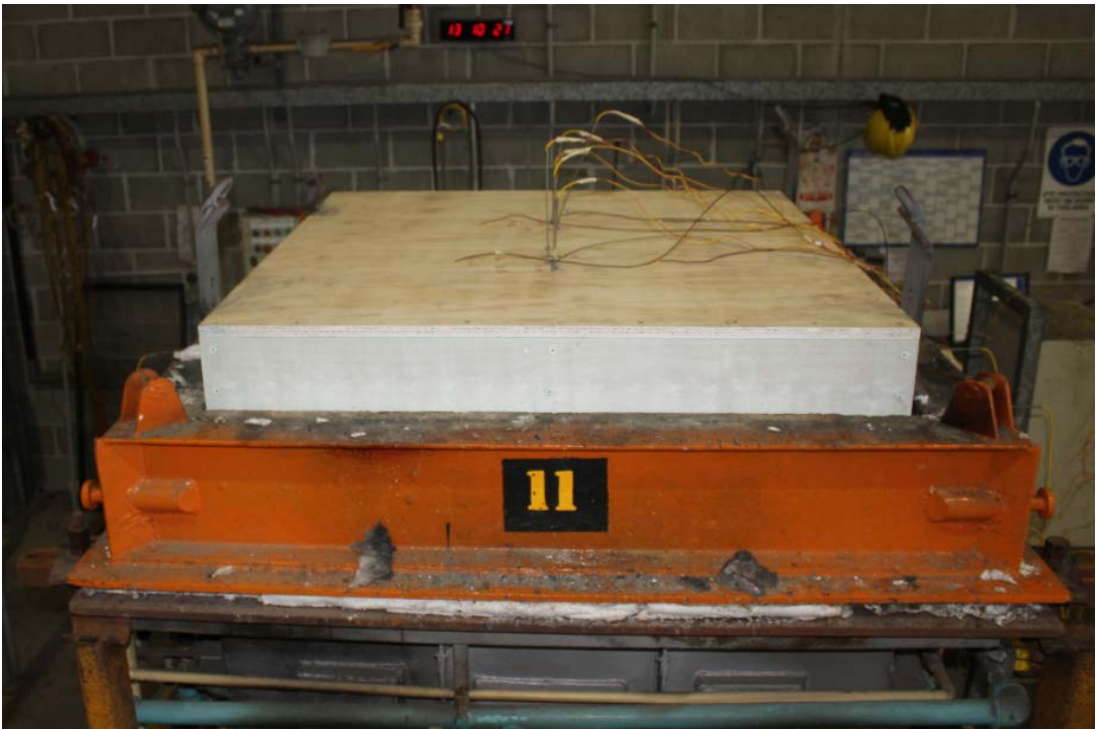
PHOTOGRAPH 2 – UNEXPOSED FACE OF SPECIMEN PRIOR TO TESTING
