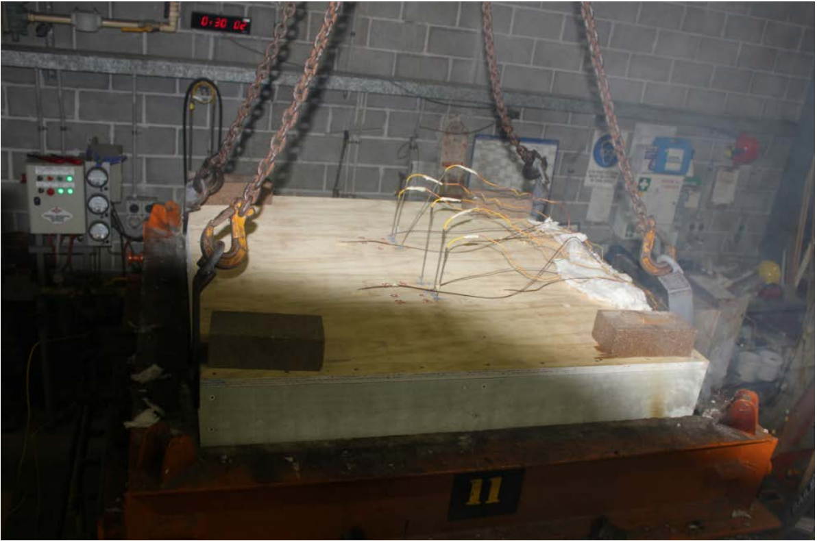
PHOTOGRAPH 3 – SPECIMEN AFTER 30 MINUTES OF TESTING
