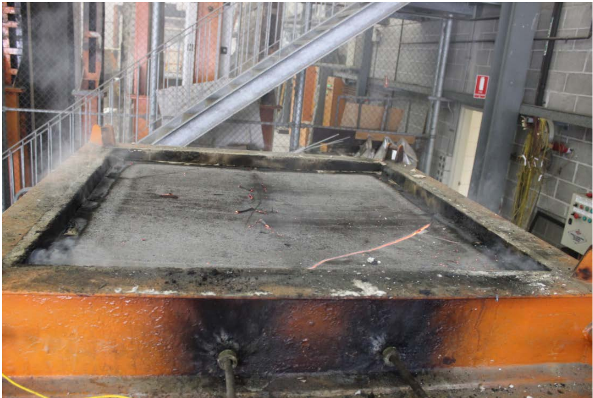
PHOTOGRAPH 8 – VILLABOARD FROM THE EXPOSED FACE OF SPECIMEN AT CONCLUSION OF TESTING
