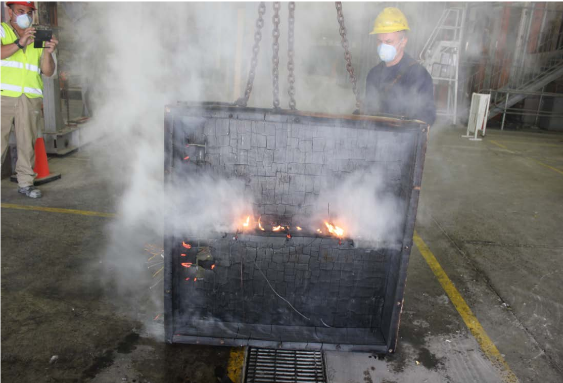
PHOTOGRAPH 10 – EXPOSED FACE OF SPECIMEN AT CONCLUSION OF TESTING
