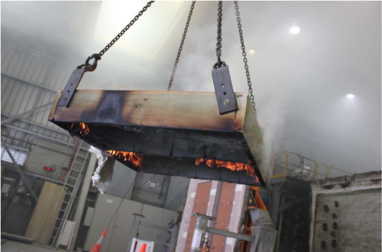
PHOTOGRAPH 9 – EXPOSED FACE OF SPECIMEN AT CONCLUSION OF TESTING
