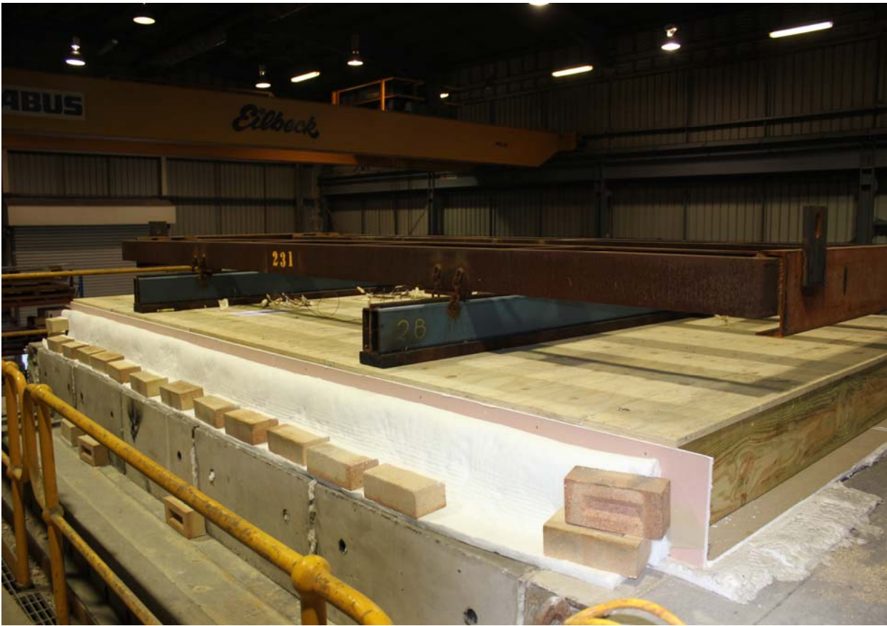
PHOTOGRAPH 2 – UNEXPOSED FACE OF THE SPECIMEN PRIOR TO LOADING
