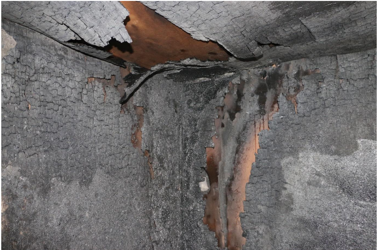
Photograph 32: After test - above burner
